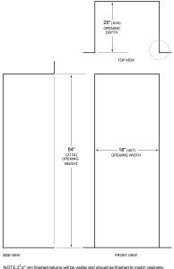
NOTE:3<sup>1</sup>/<sub>2</sub>" (89) finished returns will be visible and should be finished to match cabinetry
