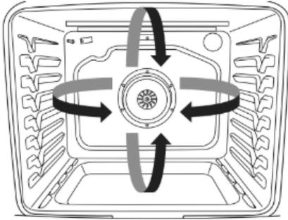
During convection cooking, the bake and broil burners and convection element cycle on and off in intervals to maintain the oven temperature, while the fan circulates the hot air.
